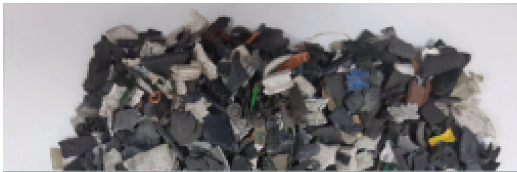
Shredded plastic from telecom equipment
