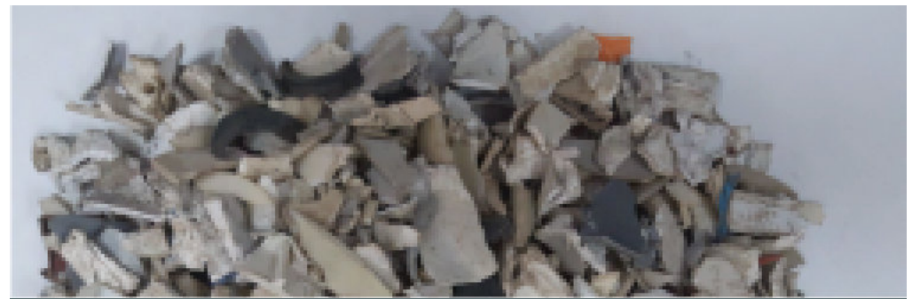
Shredded plastic from washing machines
