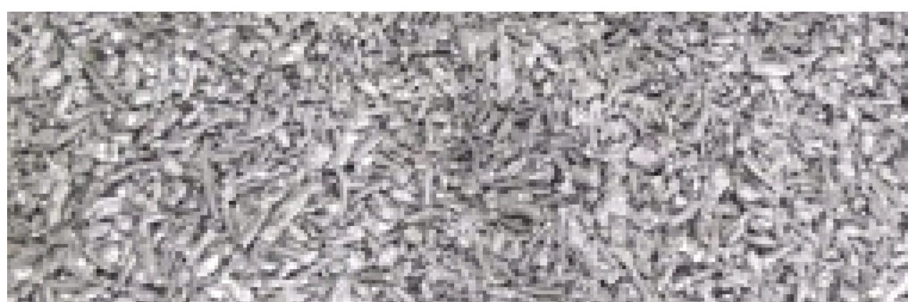
Aluminum from cables (TALL)
